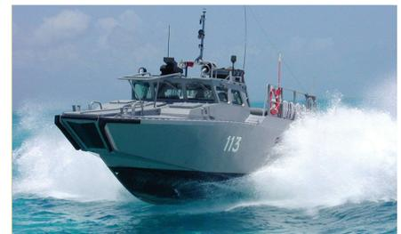
*Depending on the mission, the Riverine Command Boat can bristle with weapons from six different mounts. It has a remote-controlled weapon mount for a .50-caliber machine gun — or other weapon — on a mast behind the cockpit. It will also have a twin weapon mount on the bow that is controlled from the cockpit, as well as four mounts for crew-served weapons elsewhere on the boat. The mounts include electrical power supply to allow the use of mini-guns.*
