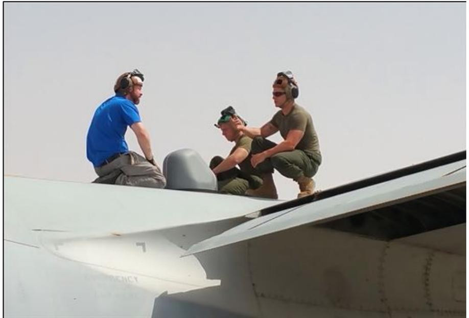
A Marine-contractor team installs the Hatch-Mounted Satellite Communication Antenna System onto the fuselage of a C-130 Hercules aircraft. HMSAS provides secure voice, tactical classified network access, common tactical picture, secure chat and streaming intelligence and reconnaissance video for commanders in the field.
