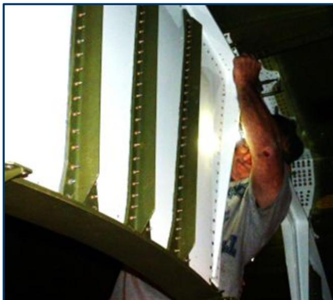
David McLemore, sheet metal mechanic, installs web plates on the Batman fitting. The fitting gets its nickname due to its resemblance to the cowl worn by the fictional character. U.S. Air Force photo by Isaac Cruz
