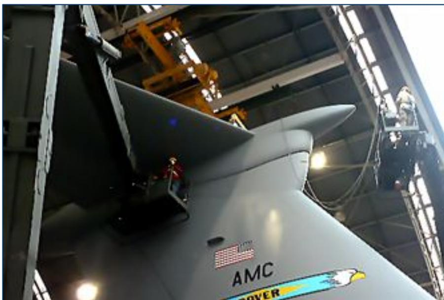
Flight control mechanics install the tail on a C-5M. The Warner Robins Air Logistics Complex will be completing a new retrofit on 51 C-5s between now and 2020. U.S. Air Force photo by Isaac Cruz
