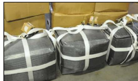
The Enhanced Speed Bag System, or ESBS, is a low-cost, materiel technology solution developed by NSRDEC and ARDEC that uses padded cargo bags, which help increase the survivability of Class V munitions up to 98 percent during aerial re-supply missions and provides small units with an organic, rapid resupply capability. (U.S. Army photo by NSRDEC Public Affairs)
